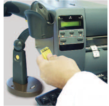
A cassette is scanned at a cutting station into the ScanPrint system to print slide labels. The ScanPrint system does not require a PC workstation to process data and print labels. All data management is performed by the intelligent printer.
