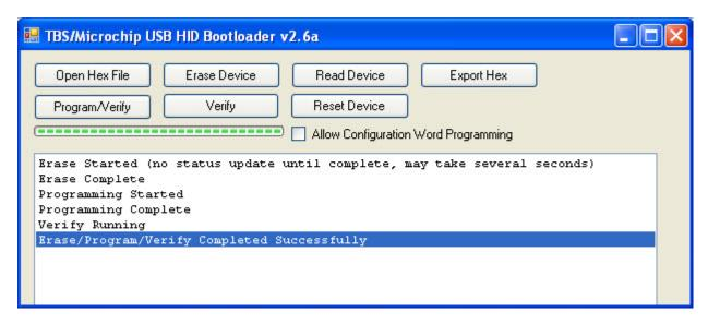
7. Click the "Reset Device" button in the bootloader software or reset the waterbath by turning the main power switch off then on. Verify the correct model and firmware version are displayed on the LEDs during reset.
