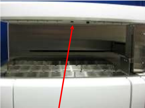
Push button to release the bezel
