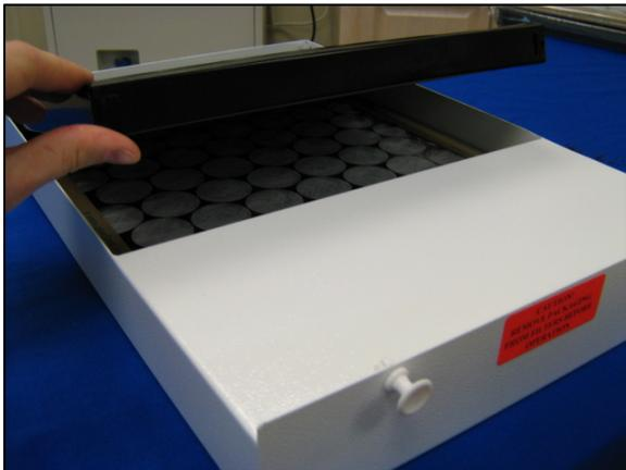
**3.4.1.3 Ensure that catch pins are pulled out.**
