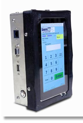
A powerful single board computer, running on open source Linux (optional Windows 10). The Smart Touch Panel is ideally suited for data collection over networks with barcode scanners, thermal printers, PLC's or as an industrial PC HMI.
